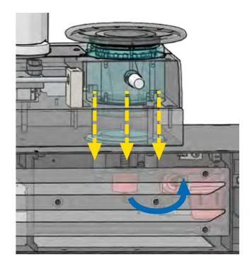
Granite is a natural material with one of the lowest thermal expansion coefficients in the world, an important peculiarity when it comes to measurement: for this reason, the E346V+ presetter machine is equipped with a **NATURAL GRANITE** base and column.
